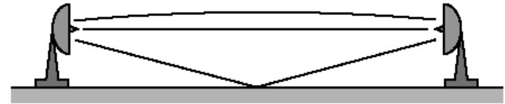
(a) Microwave line of sight
